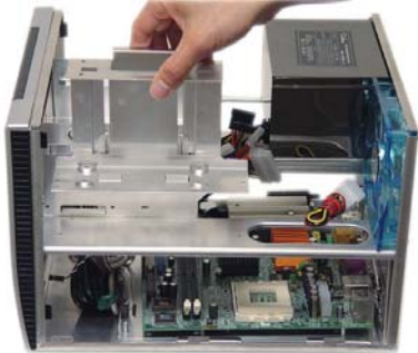
13. Pull up and take out the HDD cage.
