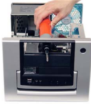
11. Once you detach the plate, Use a screw driver to knock it out.
