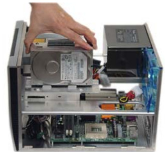
18. Put the HDD cage back.
