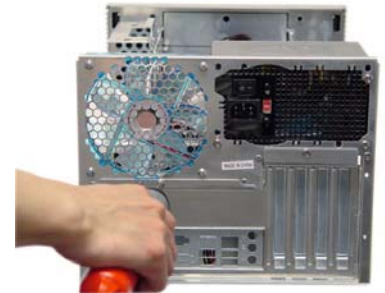
3. Unscrew the motherboard tray.
