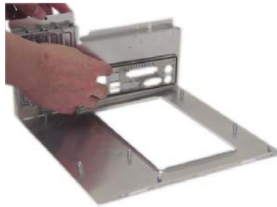
5. If your motherboard size and layout is not universal standard, then you need to remove the I/O bracket and replace with the one that comes with your motherboard.
