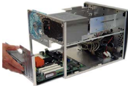
11. Push motherboard tray back to the case.
