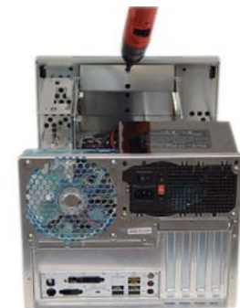
12. Remove 5.25" drive plate. It's easier to use a screw driver to pull it out a little.
