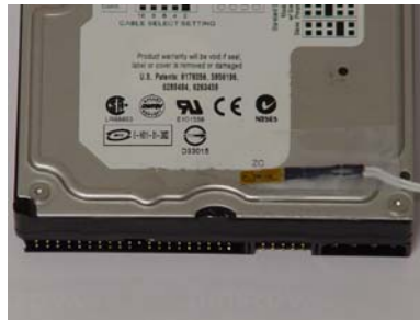
20. LCD sensors: You can tape temperature sensor on HDD to get more accurate temperature of HDD.
