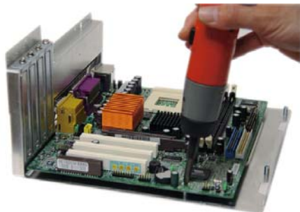
7. Screw the motherboard on motherboard tray
