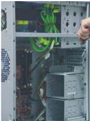
1.13 Break and remove the 3.5" drive metal plates
