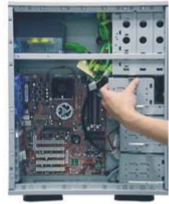
1.12 Remove the top 3.5" drive cage for external 3.5" drives.
