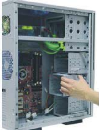
1.16 Remove 2nd 3.5" drive cage for internal drives.
