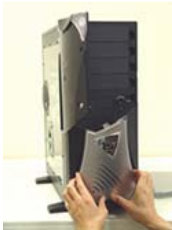
4.2.1.Open the Front Door. Insert the Bottom Mask first. Snap in bottom clip into the hole.
