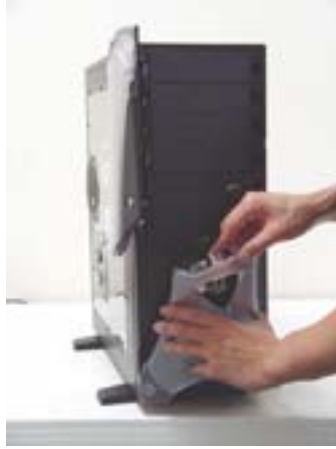
4.1.2.Pull the Mask upward to take it out.
