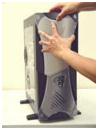
4.2.4.Close the front door to insert Upper Mask. Snap in upper clip, then the side clips.
