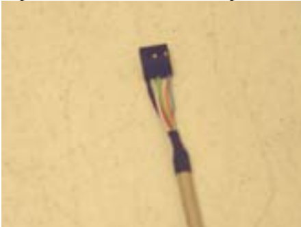
2.7.IEEE1394 Firewire cable connector (9-pin consists of 6 wires). Please refer to MB user's manual.
