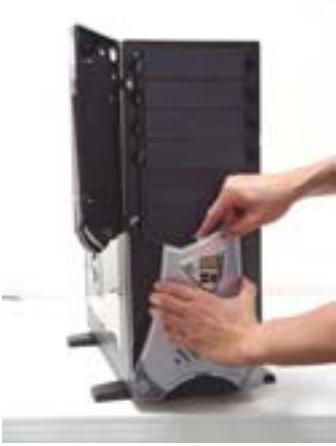
4.1.1.Open the front door. Press down the upper clip and pull out the upper part
