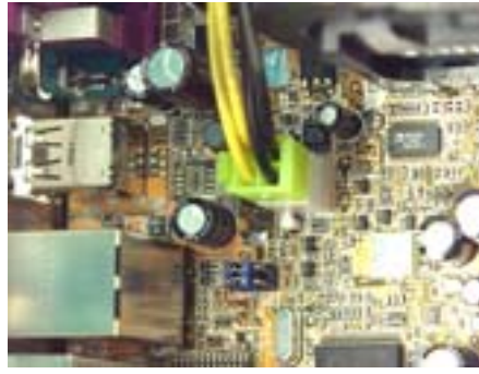
2.2.Install 4-pin cable connector to motherboard. (This is for P4 MB only) Some P4 motherboards may not need to install this. Please refer to MB manual.
