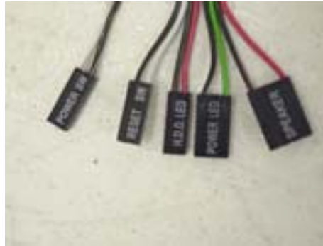
2.4.LED's and Front Panel Leads-Power SW, Power LED, HDD LED, Reset SW and Speaker.
