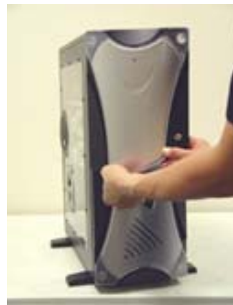
4.2.5.Once the upper and side clips are in, then snap the bottom clip in.
