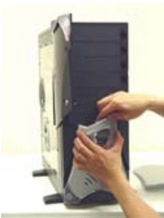
4.2.3.Push down on the upper clip to fit into the hole. Push in.
