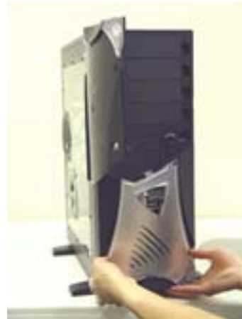
4.2.2.Then, snap in the Side Clips into the holes.
