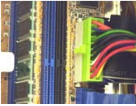
2.1.Install 20-pin cable connector from power supply to motherboard. Please refer to MB manual
