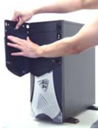
4.1.3. Press down the upper clip and squeeze the side clips from the back of the front door, then push them out.
