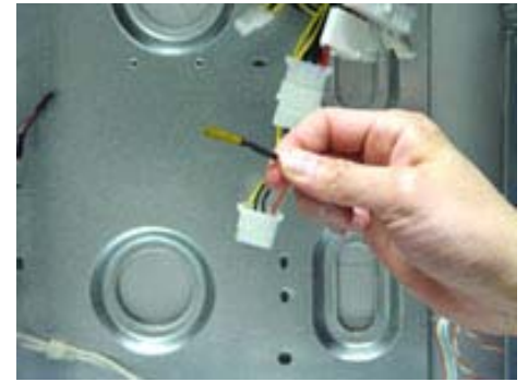
Step (3): This is the temperature sensor. It's very fragile. Be gentle. from power supply.
