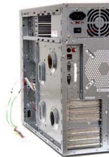
28. Install LED Lights: Find 2* LED connectors from the front Panel. They are 2*2-pin connectors that lead out to 2*4-pin connectors (1*Male, 1*Female)
