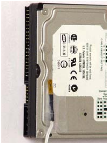
31. You can either tape the sensor on hard drive or on CPU Heat sink or leave it inside the case to get the overall system temperature.
