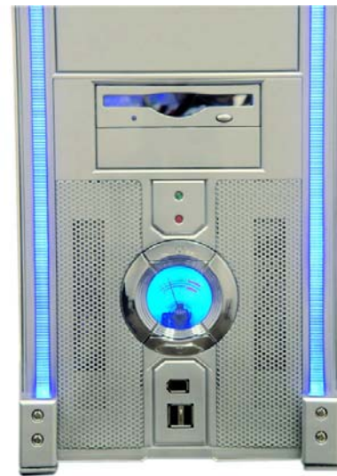
32. Once powered on, the LCD shows temperature readout with back lighting.
