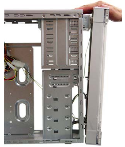
16. Put the front panel back and screw back the 4 screws to secure the front panel.
