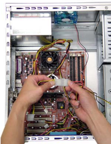
29. Connect the 4-pin Male connector to a 4-pin connector Female from power supply.
