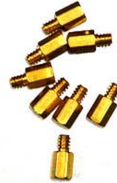
3: Find the motherboard stand-offs from the enclosed screw box.
