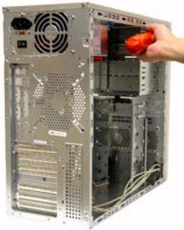
Step (4): Unscrew the other 2 screws from the other side.
