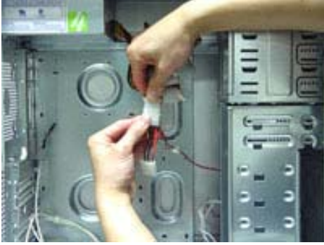
Step (1): Connect 4-pin Male connector from LCD to a 4-pin Female connector from Power Supply.
