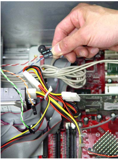
23. Find "HDD LED" and "Reset SW" cables.
