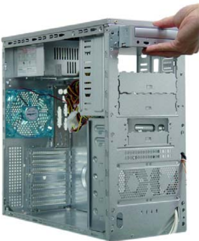
11. Force out the 5.25" metal plate from inside with a screw driver, then insert 5.25" drive.
