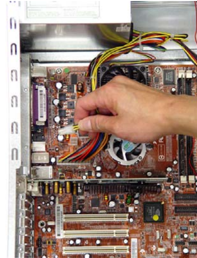
19. Find the 4-pin P4 connector from power supply. (for P4 only) If you have AMD or P3 board, You do not need to connect it.
