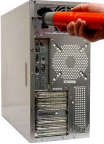
Step (1): Unscrew both side panels
