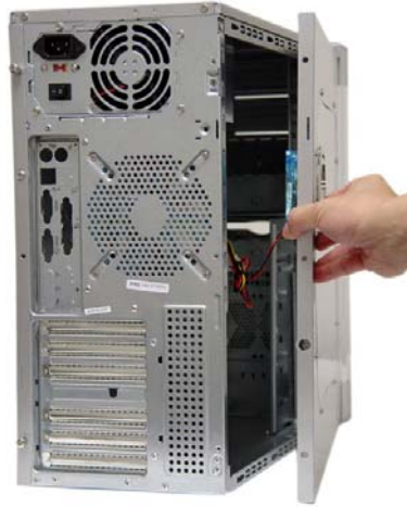
2. Pull the side panel back then pull out.
