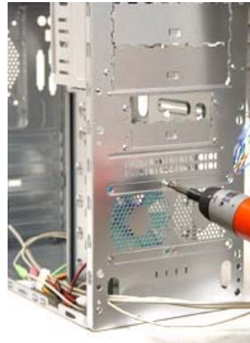
10. Front Case Fans (Optional): You can put up to 2*80mm fans in the front.
