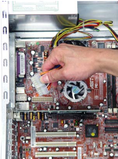
17. Find the 20pin/or 24pin main connector from Power Supply.
