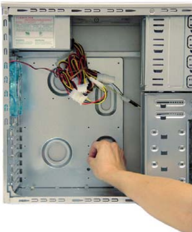
4: Put the motherboard stand-offs on the motherboard tray.
