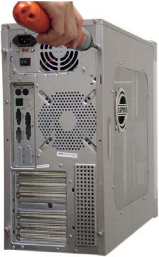
1: Unscrew the thumb screws from Side Panel.
