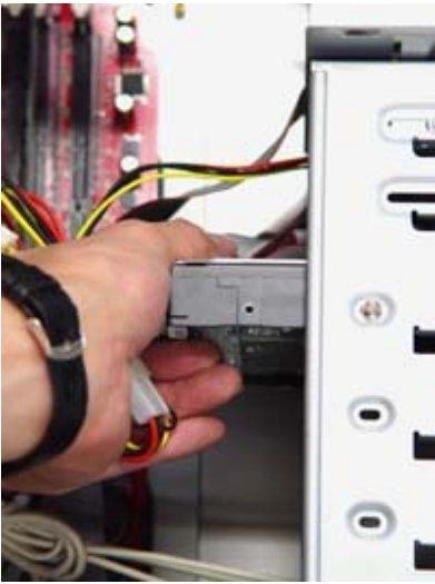
14. 3.5" Internal Drives: Install 3.5" hidden drivers such as hard drive and zip drive.
