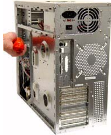
Step (3): There are 4 screws that hold the front panel to the case. (2 on each side) Unscrew 2 screws from the back of front panel on one side.
