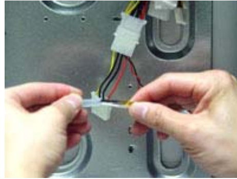
Step (2): Remove the protective plastic tube from the sensor.
