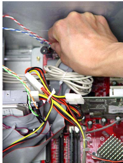
28. Find "Power SW" and "+P LED" "-P LED" cables and plug onto M/B. Please refer to M/B user manual.
