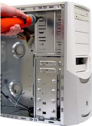
14. Secure the 5.25" drives in place with screws.
