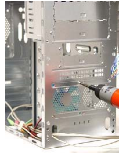
10. Optional: Install case fan in the front panel (You can put up to 2*80mm fans). Then screw the front panel back.
