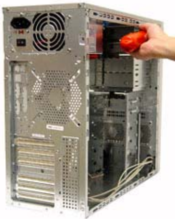
Step (4): Unscrew the other 3 screws from the other side.
