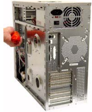
Step (3): There are 6 screws hold the front panel to the case. Unscrew 3 screws at one side from inside of the case.
