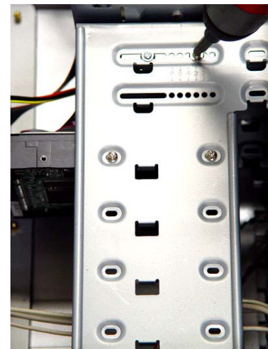
16. Slide in 3.5" drives and secure in place with screws.
