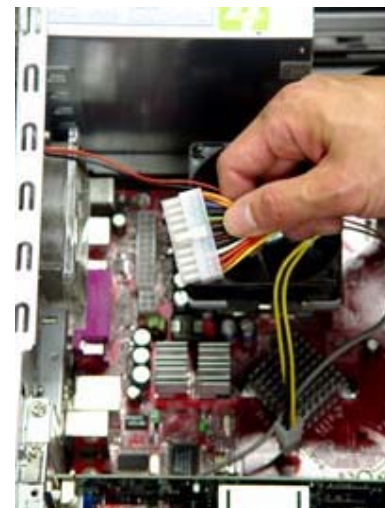
20. Find the 20-pin main power connector from power supply.
