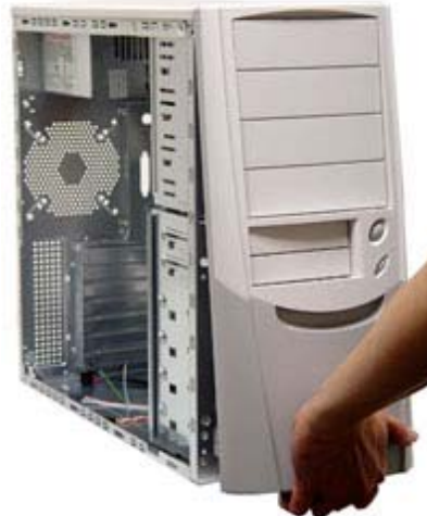
Step (5): Pull out the front panel from the bottom.
