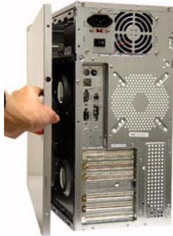
Step (2): Take out the side panel (motherboard side)
