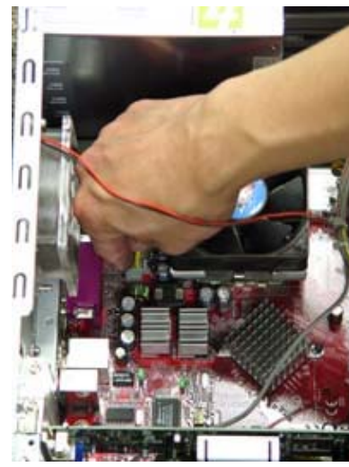
23. Plug into motherboard. (for Intel P4 motherboard only)
