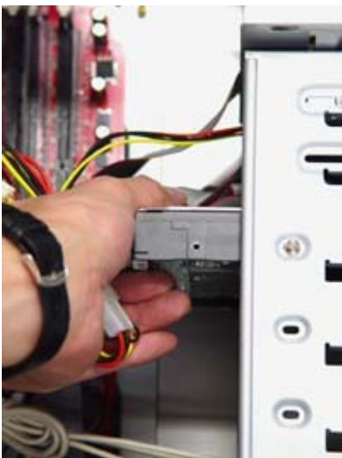
17. Install 3.5" hidden drives such as hard drive, zip drive.
