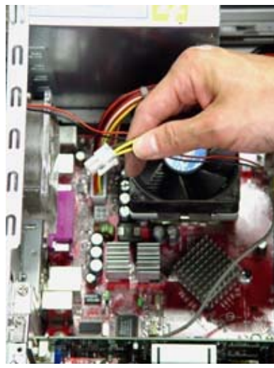
22. Find the 4-pin P4 connector from power supply. (for P4 only)
