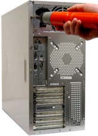
Step (1): Unscrew the side Panel (motherboard side)
