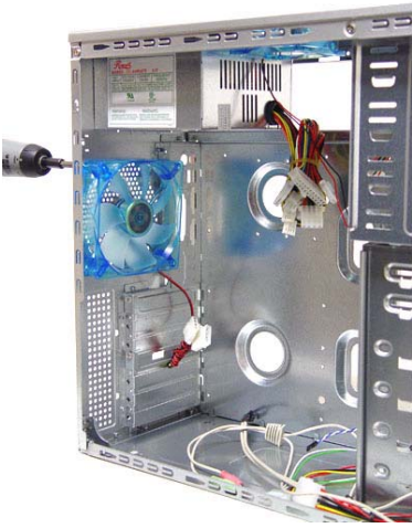
11. Optional: Install case fan at rear (1*80mm-120mm fan)
